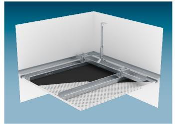
Cleaneo UFF plaster base boards with fleece or foil lamination on the rear side are screw fastened to a metal grid of carrying and furring channels (double-layer profiles) made of sheet metal profiles CD 60/27. Anchoring of the CD channels is undertaken with suspenders on the basic ceiling. An acoustically effective insulation layer can be laid upon the furring channels.
